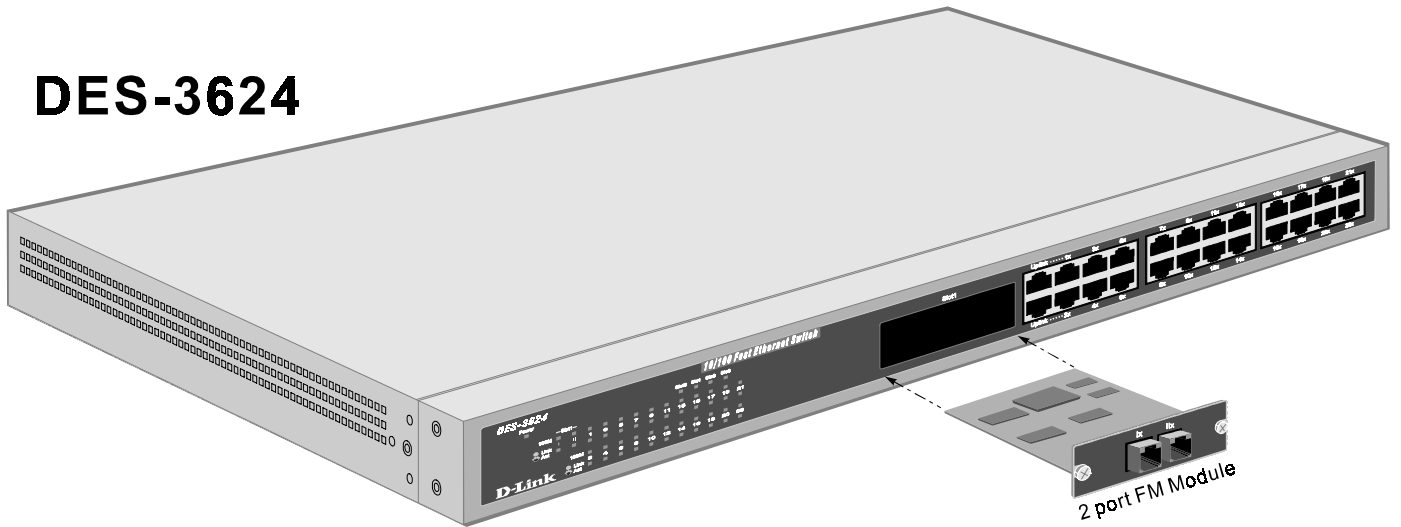
Figure 3-6. Two-port, 100BASE-FX (MT-RJ) module
